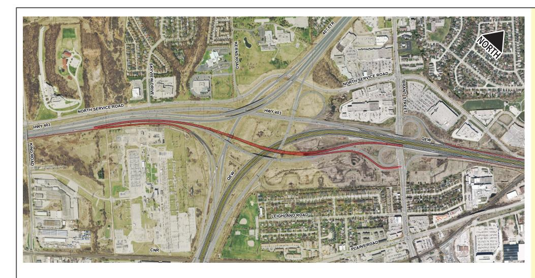
Highway 403 is widened by one General Purpose Lane (GPL) in each direction by widening into the median.
