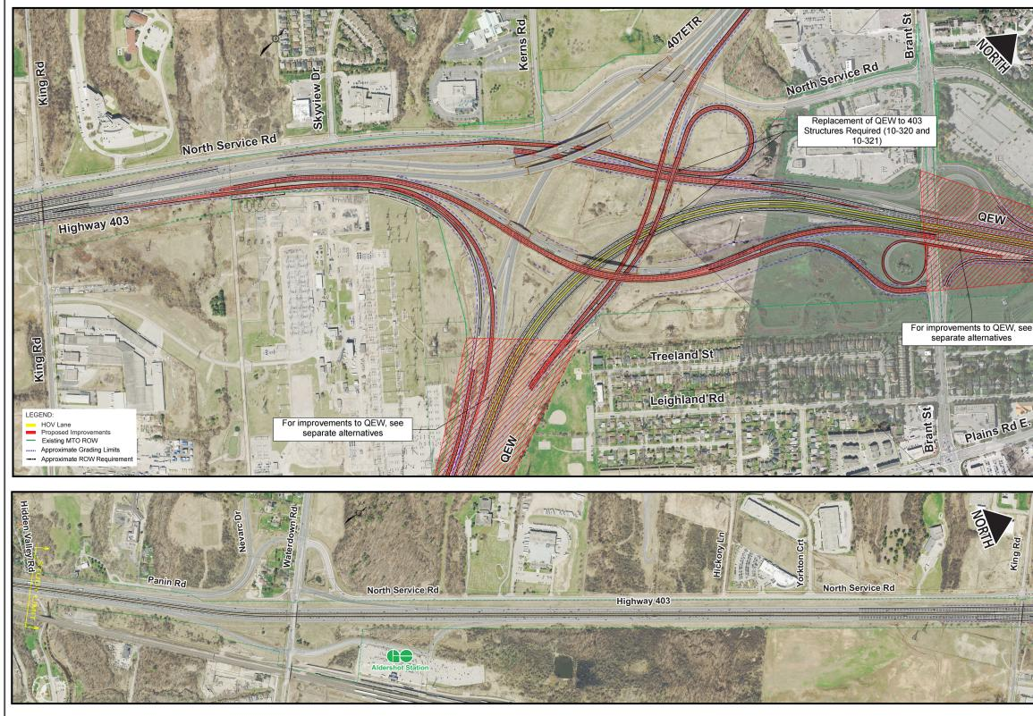
In all alternatives, Highway 403 is widened by one General Purpose Lane (GPL) in each direction by widening into the median.
