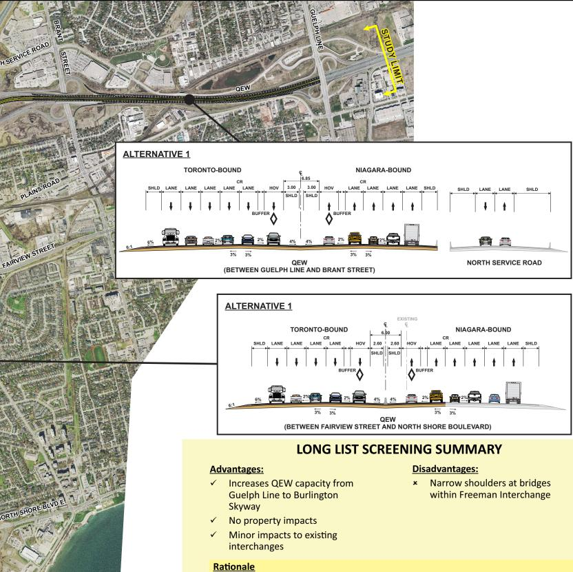
Carried forward as a viable alternative for having low construction cost, simple construction staging, and minimal property and natural impacts.
