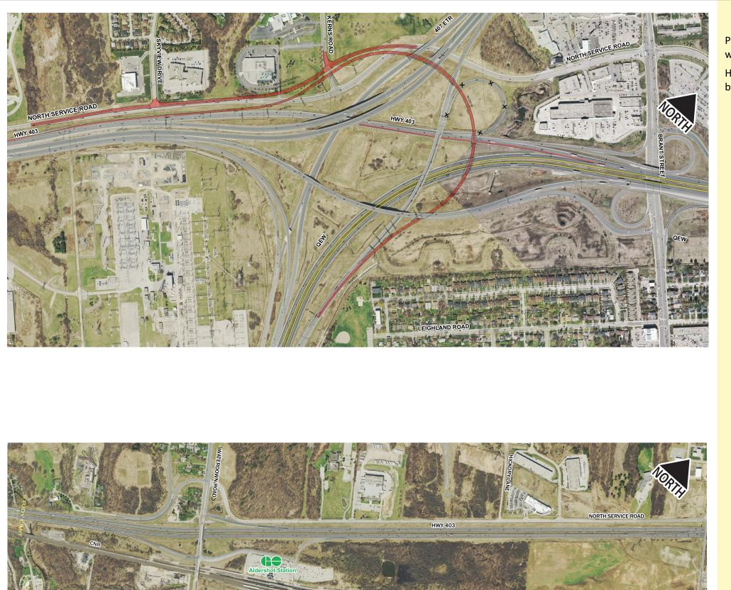
Provide a new semi directional ramp for the QEW northbound to Highway 403 westbound ramp.
