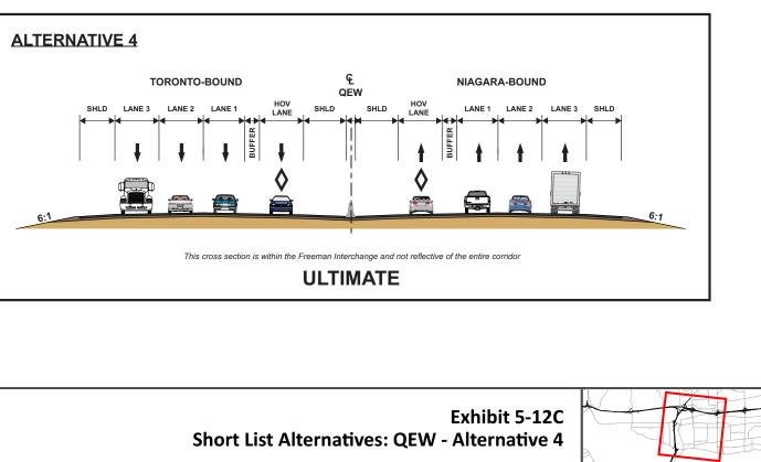
• In Alternative 4, the QEW is widened into the median as well as the outside resulting in a larger footprint. This accommodates an HOV lane as well as a General Purpose Lane in each direction between Guelph Line and the Burlington Skyway.
